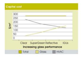
The chart shows how the investment in a high performance glass (solar and thermal insulation) reduces the capital cost of the heating and air-conditioning plant (HVAC) by reducing the building's heating and cooling loads. Running costs are reduced and savings continue for the life of the building, (source Lincoln Scott, Feb 1995).
